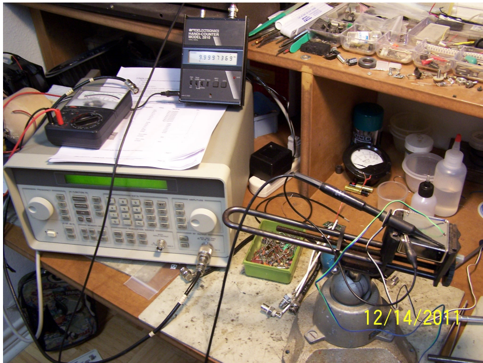
Photo 1. The oscillator frequency was measured using a frequency counter. The master clock in an HP 8647A signal generator was used as a reference.
