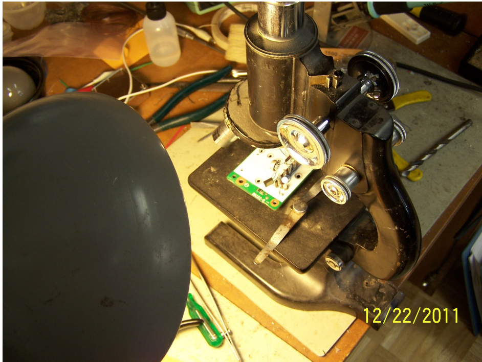
Photo 3. Checking the PWB structure using a microscope. If this had been a multi-layer board, it would have been necessary to make sure each exposed layer of copper was cleanly cut and to passivate the exposed layers with lacquer or epoxy.
