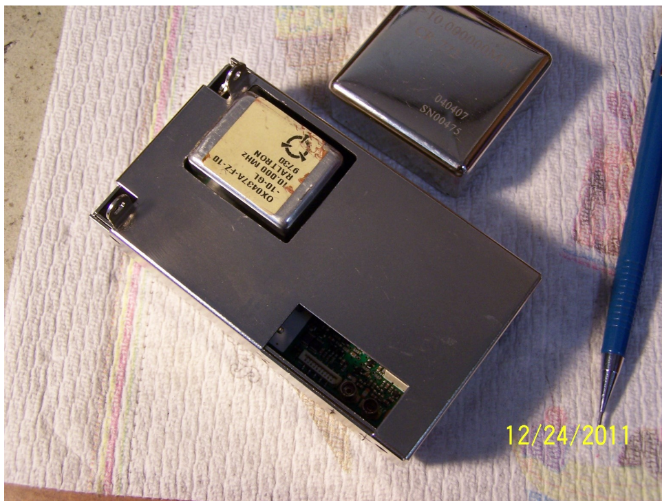
Photo 5. The oscillator module with modified cover installed. The original oscillator is visible next to the module. Coax and ribbon cable connections are made through the smaller opening in the cover.
